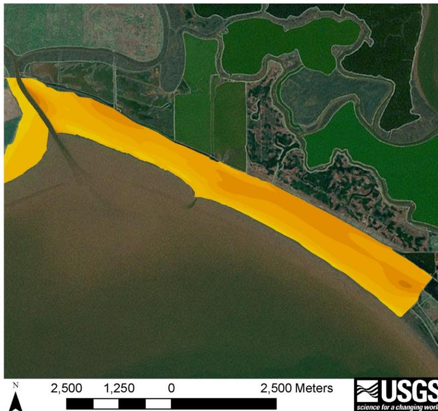
**Figure L-5.** Elevation model (3-m resolution) developed from ground RTK GPS elevation data for east San Pablo.
