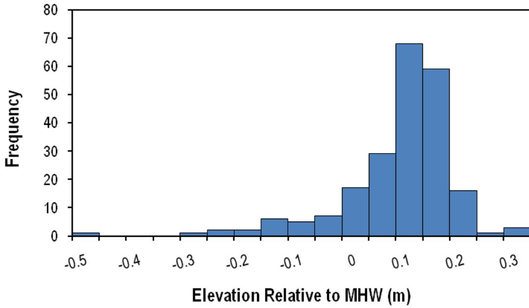
**Figure I-2.** Distribution of elevation samples relative to local mean high water (MHW) at Gambinini marsh.
