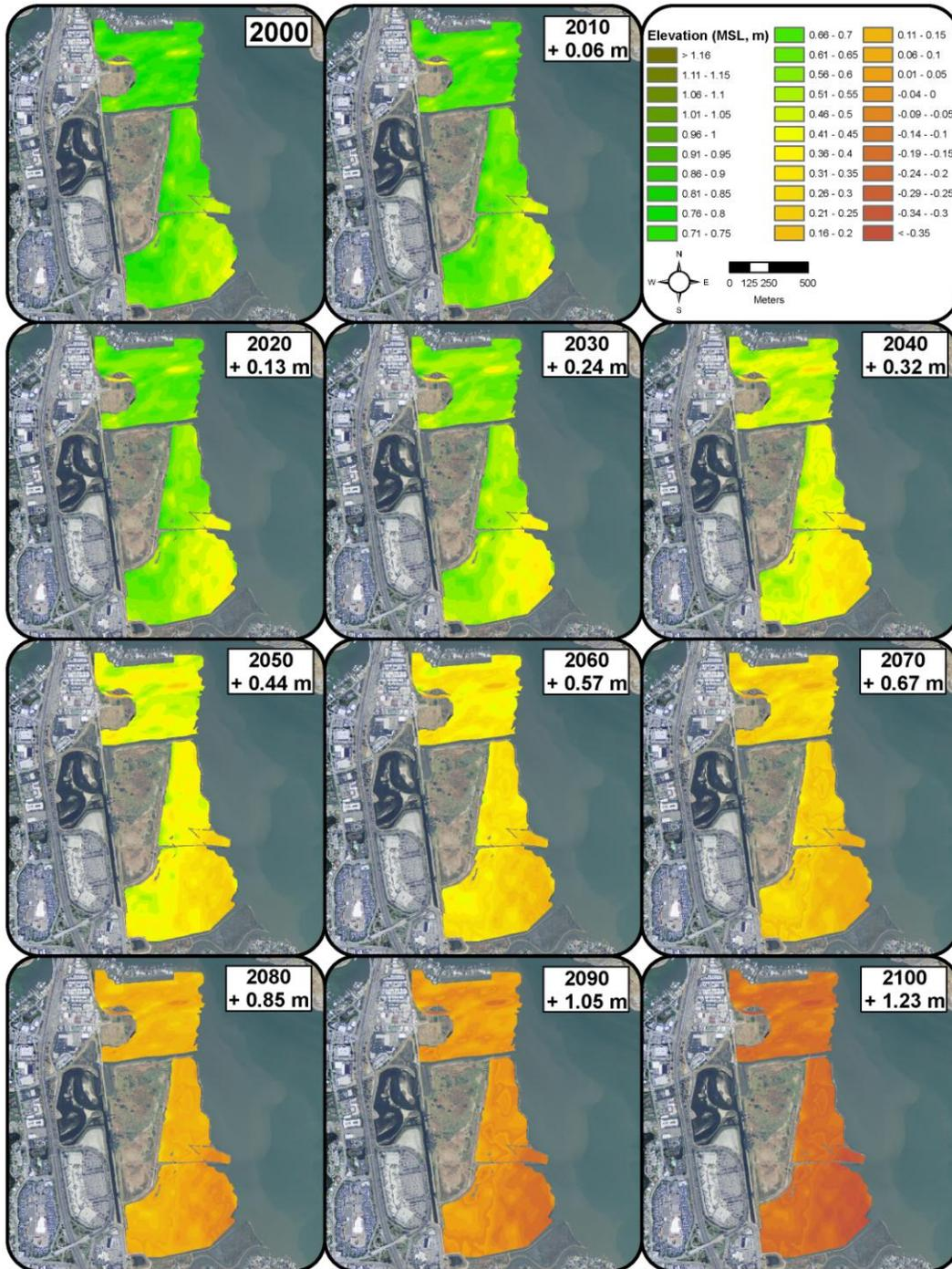
**Figure G-6.** WARMER results for Corte Madera. WARMER accounts for changes in relative seal-level, subsidence, inorganic sediment accumulation, above/below ground organic matter productivity , compaction, and decay. Non-linear sea-level rise projections for California were used (Cayan *et al.* 2009).
