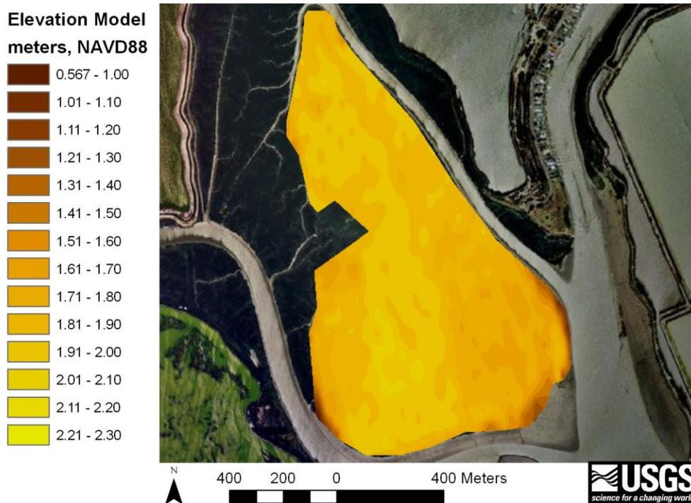
**Figure F-3.** Elevation model (3-m resolution) developed from ground RTK GPS elevation data.
