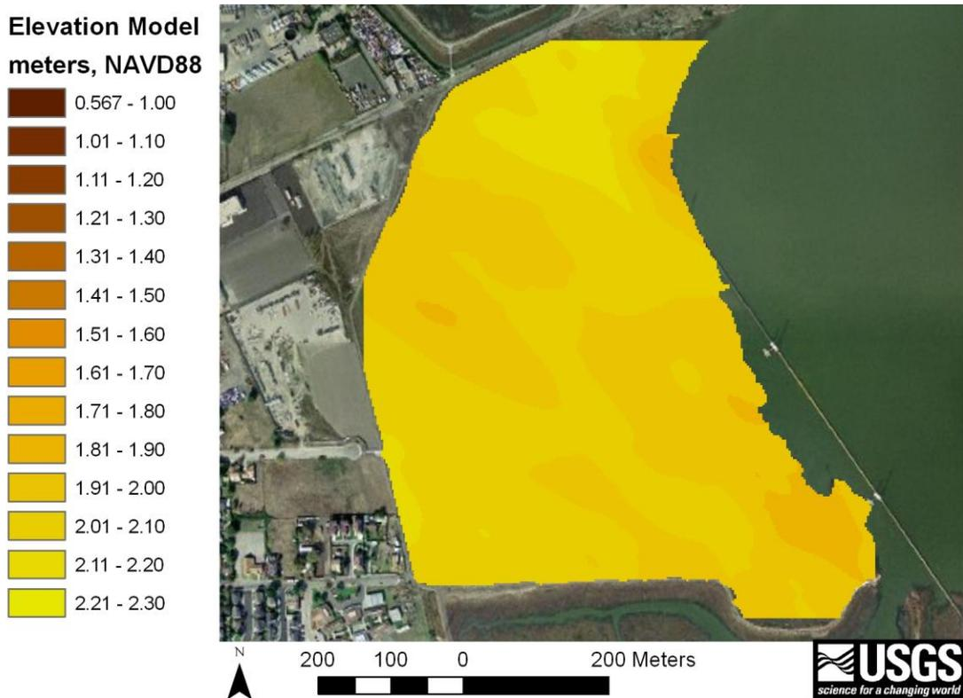
**Figure J-3.** Elevation model (3-m resolution) developed from ground RTK GPS elevation data.
