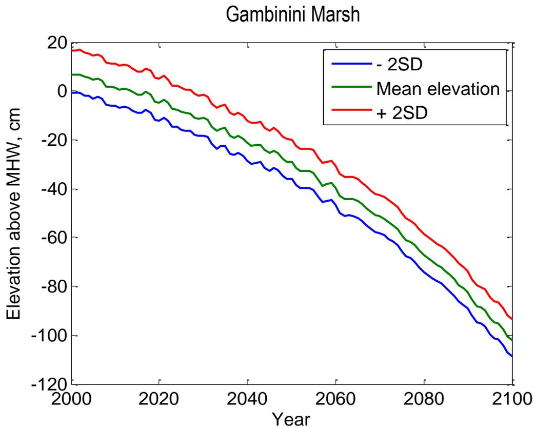
**Figure I-7.** Modeled scenarios of marsh elevation change for Gambinini. Elevation above MHW is plotted versus model year.
