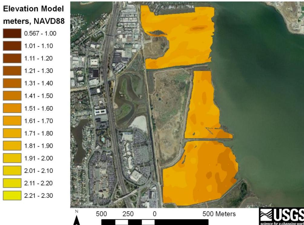
**Figure G-3.** Elevation model (3-m resolution) developed from ground RTK GPS elevation data.
