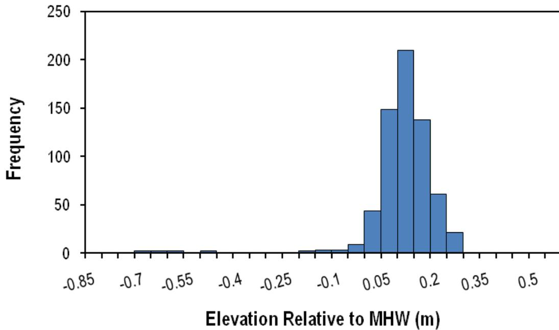
**Figure K-2.** Distribution of elevation samples relative to local mean high water (MHW) at Petaluma Marsh.
