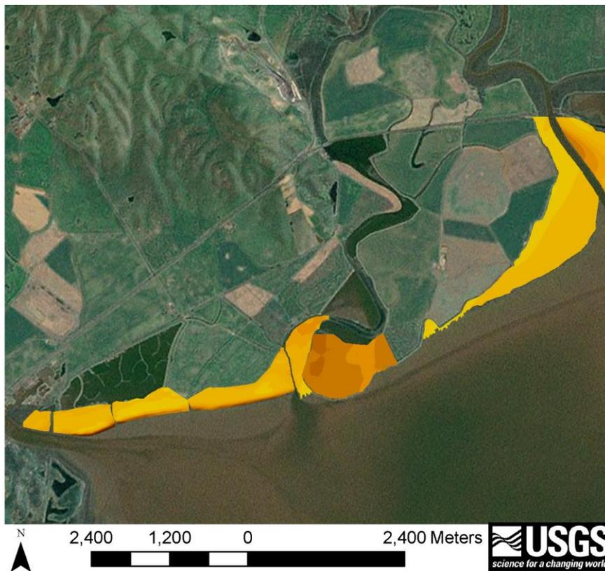
**Figure L-4.** Elevation model (3-m resolution) developed from ground RTK GPS elevation data for west San Pablo.
