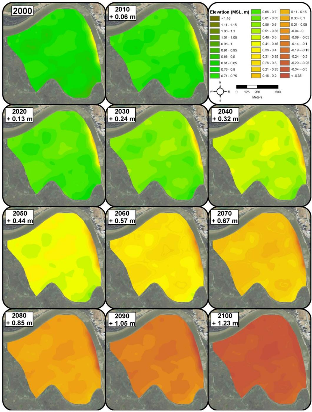
**Figure K-6.** WARMER results for Petaluma marsh. WARMER accounts for changes in relative seal-level, subsidence, inorganic sediment accumulation, above/below ground organic matter productivity , compaction, and decay. Non-linear sea-level rise projections for California were used (Cayan *et al.* 2009).
