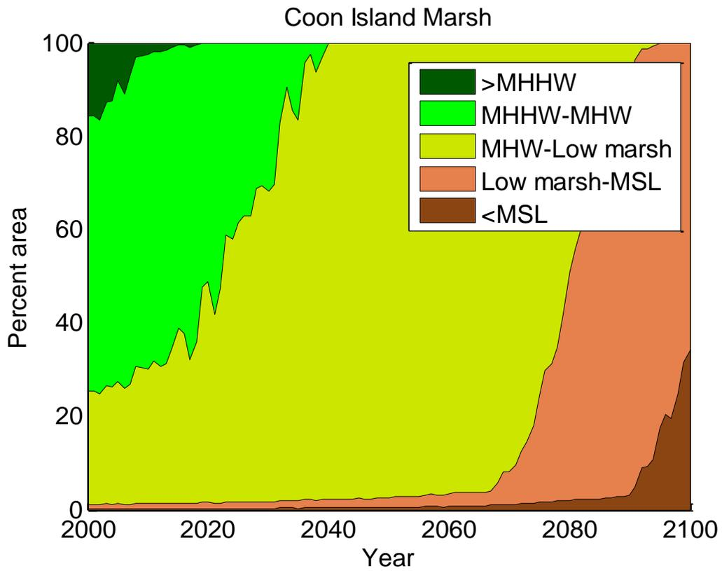
**Figure F-8.** Area of Coon Island within a given tidal range for the duration of the simulation period.
