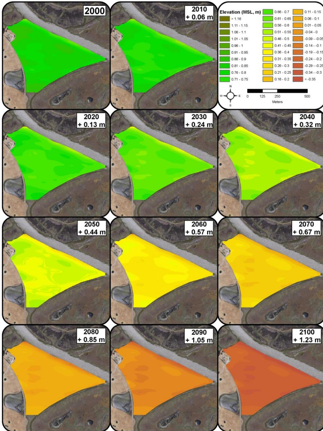
**Figure I-6.** WARMER results for Gambinini. WARMER accounts for changes in relative seal-level, subsidence, inorganic sediment accumulation, above/below ground organic matter productivity, compaction, and decay. Non-linear sea-level rise projections for California were used (Cayan *et al.* 2009).
