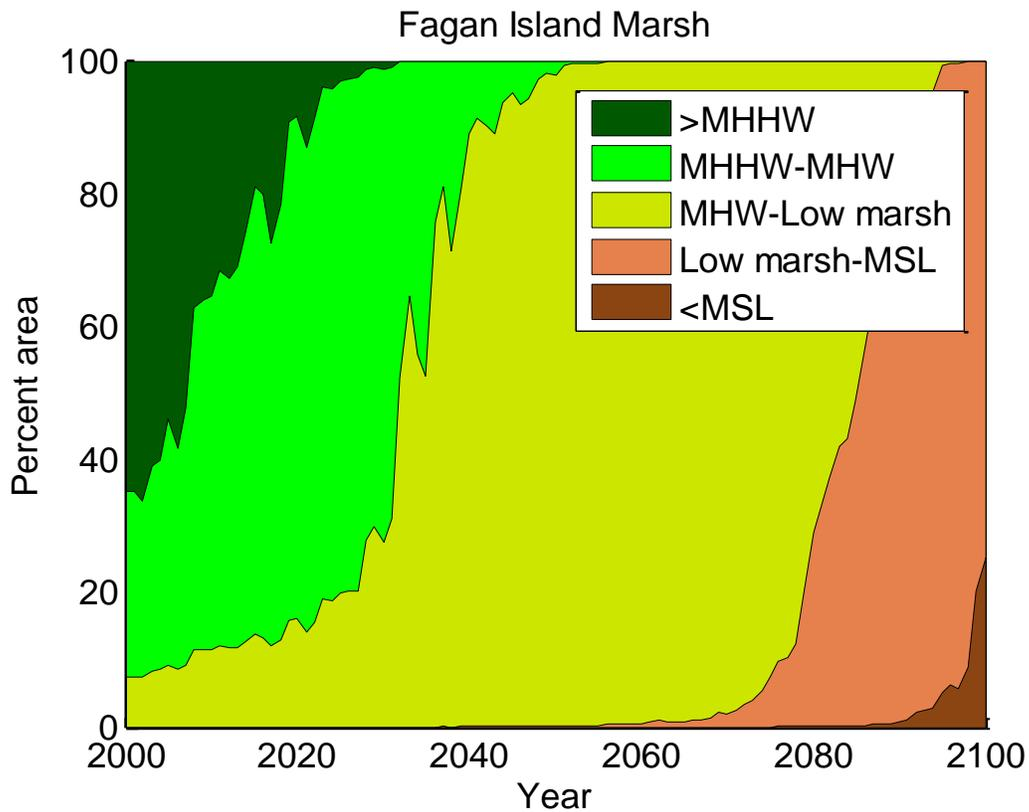
**Figure H-8.** Area of Fagan within a given tidal range for the duration of the simulation period.
