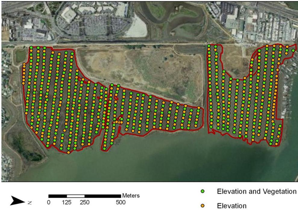
**Figure G-1.** Corte Madera with elevation and vegetation survey points taken in 2009.
