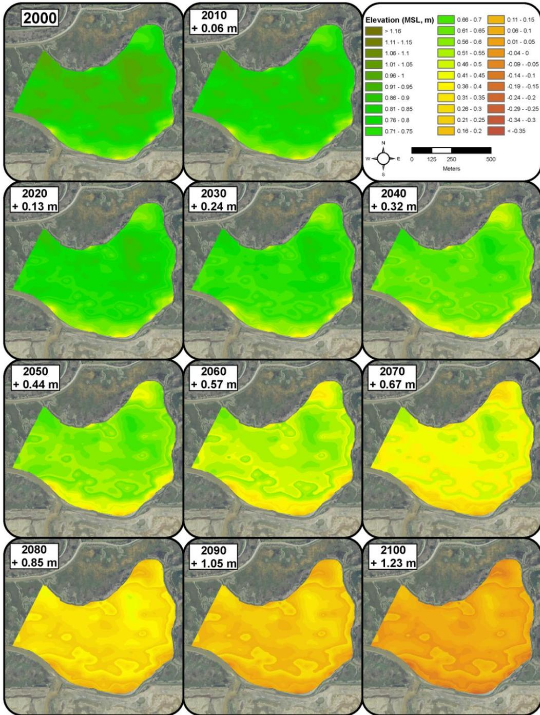
**Figure H-6.** WARMER results for Fagan. WARMER accounts for changes in relative seal-level, subsidence, inorganic sediment accumulation, above/below ground organic matter productivity, compaction, and decay. Non-linear sea-level rise projections for California were used (Cayan *et al.* 2009).
