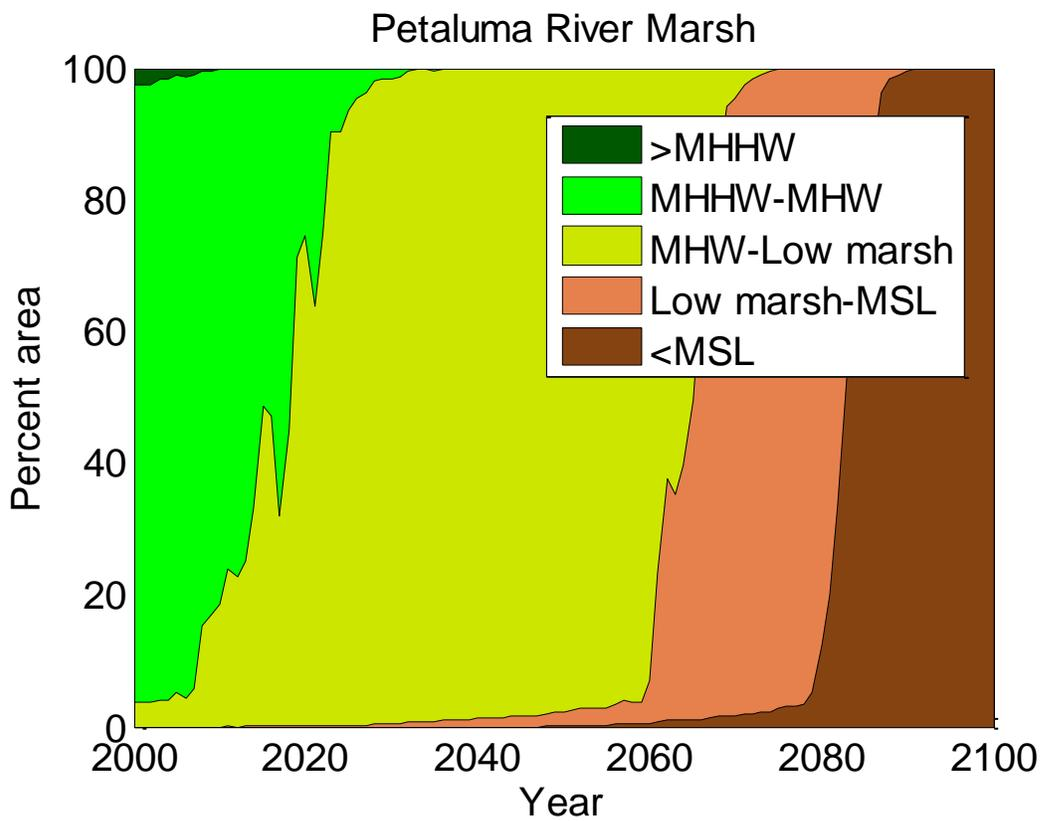
**Figure K-8.** Area of Petaluma within a given tidal range for the duration of the simulation period.
