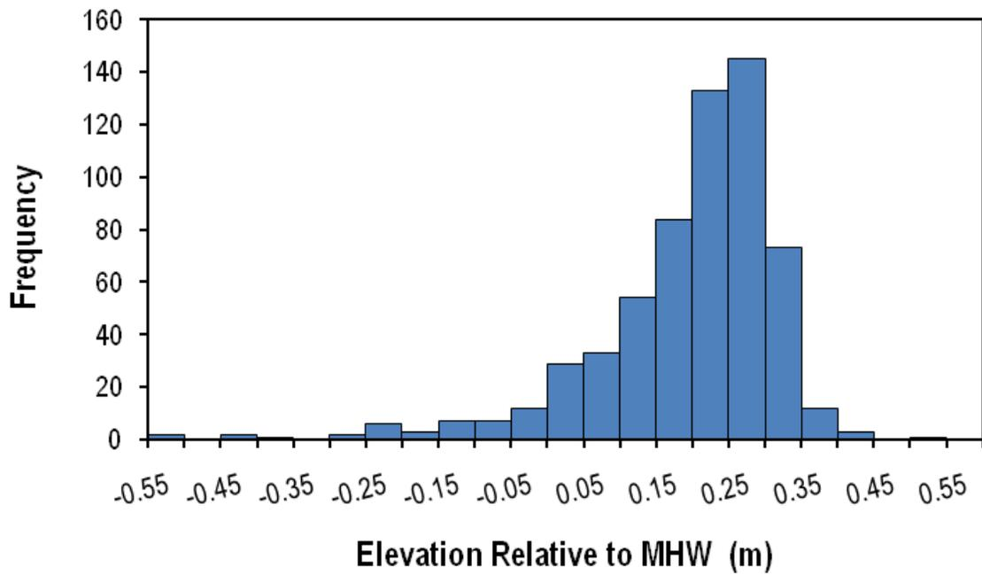
**Figure H-2.** Distribution of elevation samples relative to local mean high water (MHW) at Fagan Marsh.
