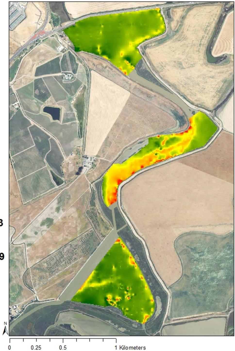
Figure 19. DEM of Tolay Creek mudflats created from 2012 bathymetric survey.
