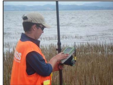
**Picture 1.** RTK GPS elevation Survey
