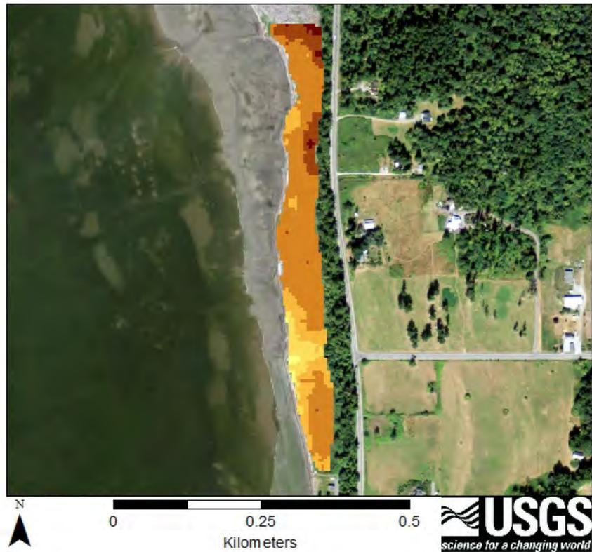
Figure A2. Elevation model (3 m resolution) developed from RTK GPS survey data.
