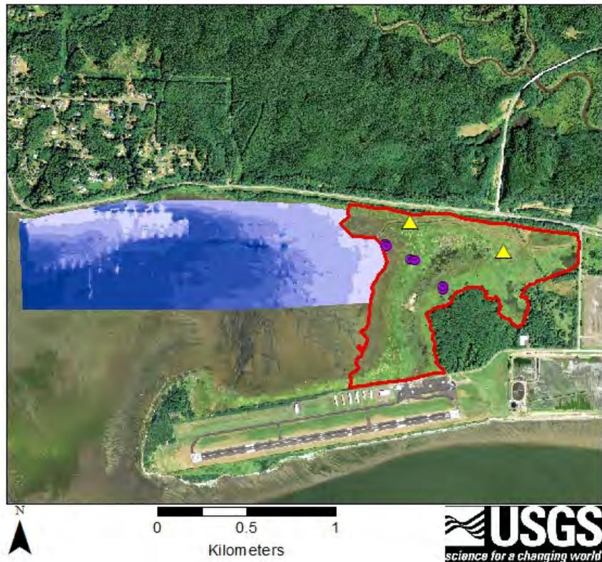
Figure E4. Near-shore bathymetry model at Grays Harbor. Water level logger and core locations are shown within the marsh study site.
