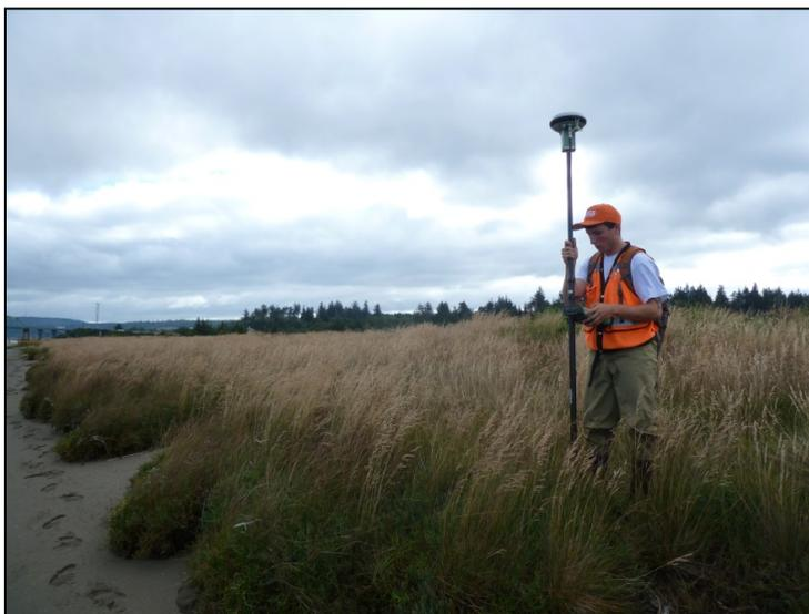
**Figure 4.** U.S. Geological Survey technician collecting elevation data using a Real-Time Kinematic Global Positioning System at Bandon National Wildlife Refuge, southern Oregon. Photograph by Katherine Powelson, U.S. Geological Survey, 2012.
