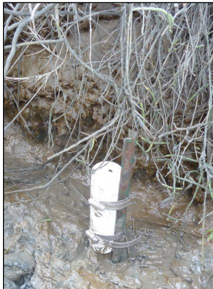
**Figure 6.** Water-level logger deployed in second-order tidal-marsh channels. Photograph by Katherine Powelson, U.S. Geological Survey, 2013.
