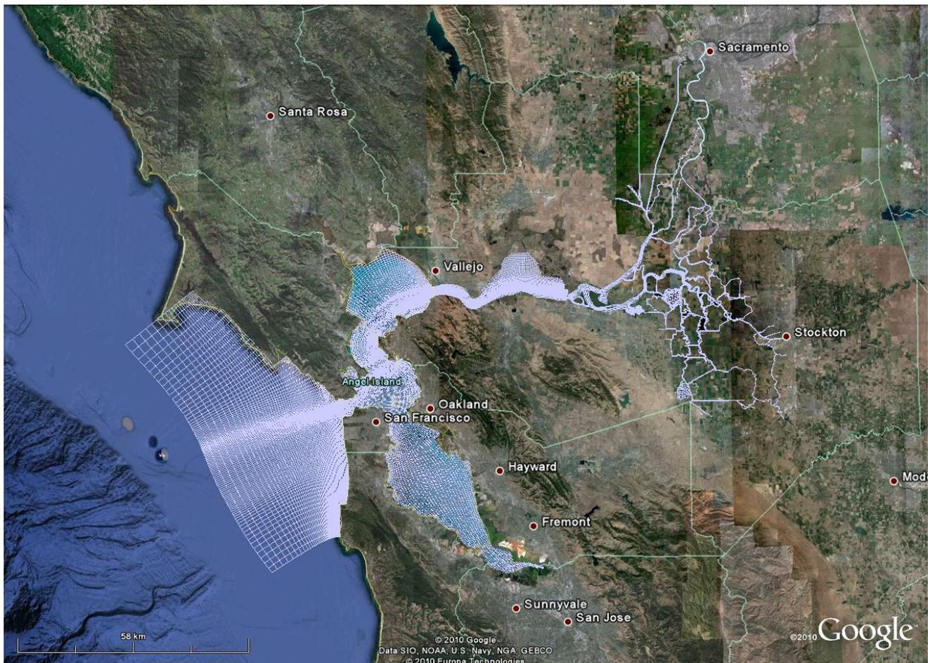
Figure 25. The Unstruc grid in the Pacific, Bay, and Delta. For more accurate modeling of habitat change in the Bay, refinement of the grid in shoals habitat is planned. A December 15, 2010 ppt presentation of the current state of development of the unstructured model is at [http://cascade.wr.usgs.gov/reports/Mick\\_vanderWegen\\_101215.zip](http://cascade.wr.usgs.gov/reports/Mick_vanderWegen_101215.zip)
