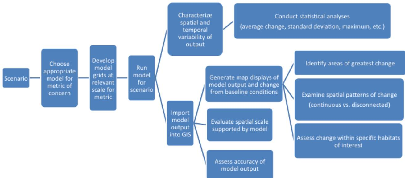
Figure 27. Flowchart for developing change metric from model output for a given scenario.
