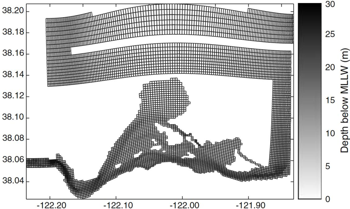
Figure 24. Ganju and Schoellhamer (2010) model grid (Fig. 2 from Ganju and Schoellhamer, 2010). Coarse grids derive from limitations in computer speed that make runs with small grid cells take days or weeks for modeling the long (decadal) time scales that are of interest. Coarse grids are typically used for modeling long time scales for large domains (e.g., Van der Wegen et al., accepted).
