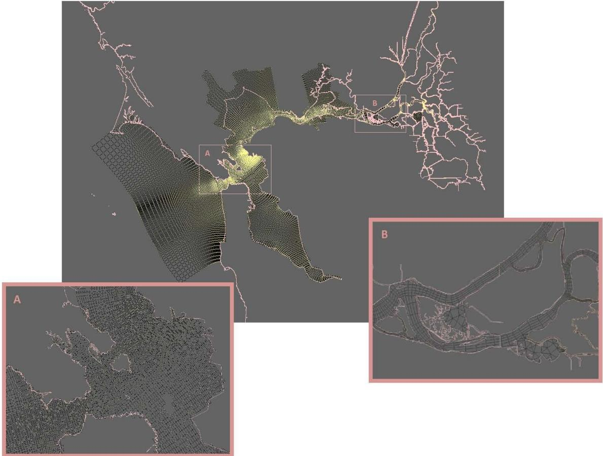
**Figure 9.** The SF Bay-Delta Delft-UNSTRUC Hydrodynamic Model incorporating a 3-dimensional hybrid grid from ocean to river.
