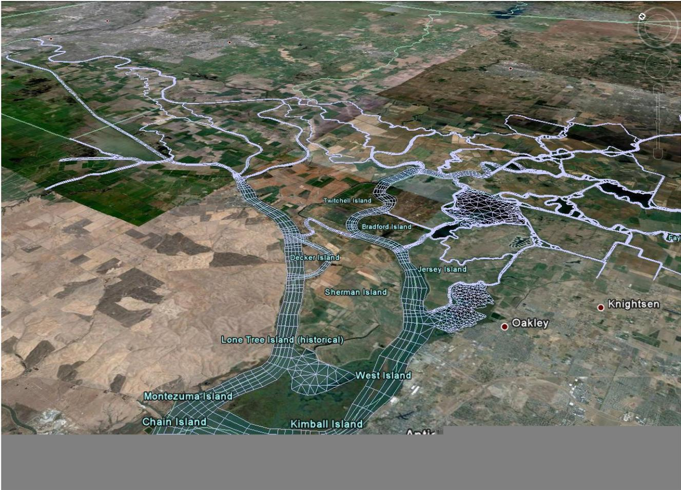
Figure 26. Example of the Unstruc grid in the Delta. The irregular polygon shapes allow computationally efficient modeling of complex geometries.
