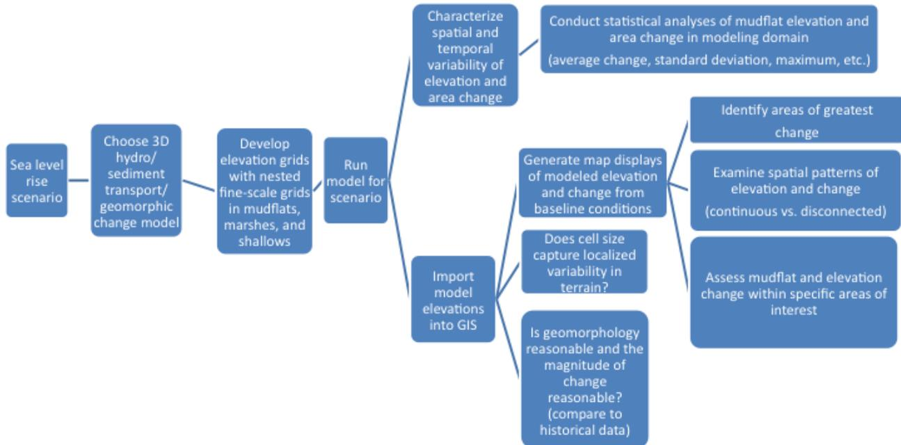
Figure 28. Flowchart for developing mud flat elevation and area change metric from model output from scenario of sea level rise
