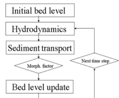
Figure 8. Flow chart of parameters in the Delft 3D sediment model
